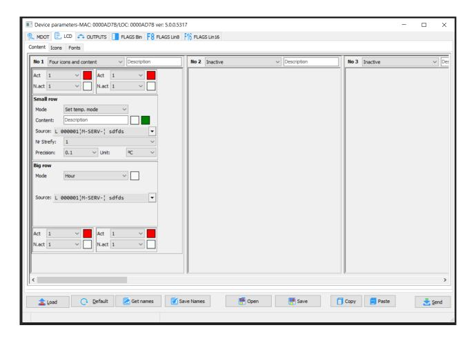
Submit the parameters by clicking *Send*. From this moment on, information from the bus about the set and current temperatures will be displayed on the LCD screen.
