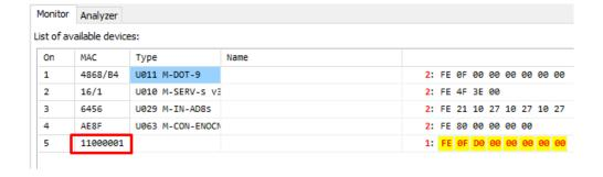
Add a new device (*Project->Add a new device manually*), entre the address, provide a name (optionally) and confirm. A new device will show on the devices list.
