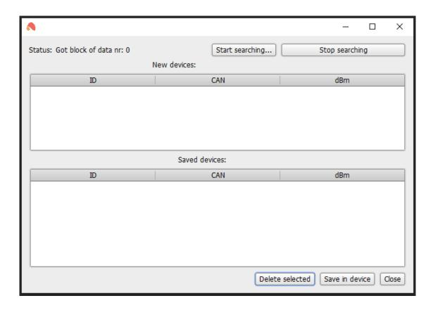
In the new window, click on *Start searching*. When the device status indicates searching, press the terminal/executive device's button. The device should show on the list of devices.
