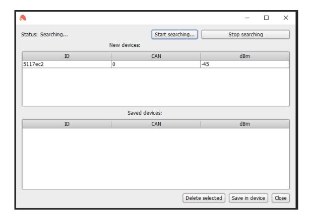
The next step is to click *Save in device* and *Close*. When you close and open the Settings again, the terminal device will appear on the list of saved devices. A change of address is only possible by editing the CAN column. Each entered change must be saved on the device with a click of a button.
