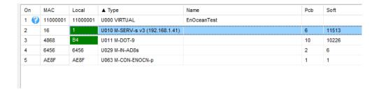
From the modules list, select the one for which you would like to create a condition and open the *Device configurator*. Choose the created virtual device as the device from which the condition is created. While creating the condition, activate the terminal EnOcean device a couple of times. This way, you will know from which input to create the condition, as the input state will change in preview.
