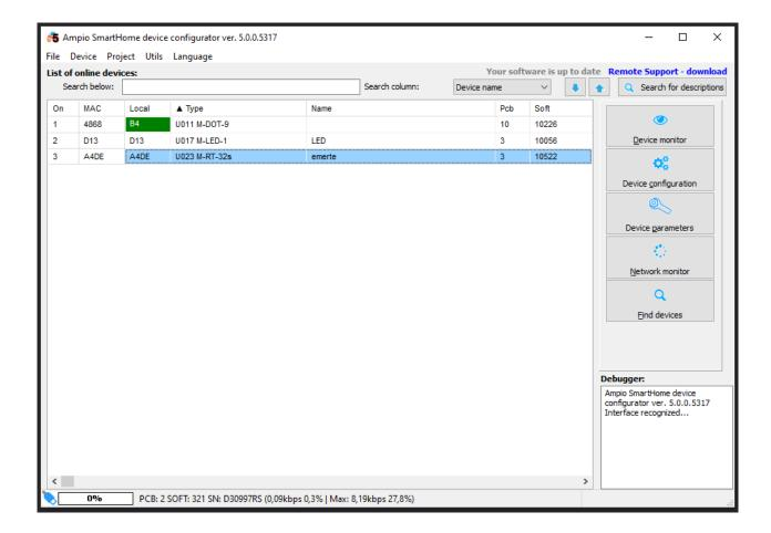
The condition is created from an M-DOT touch panel. Select the correct module on the configuration list and click Add condition from device.
