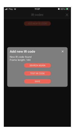
The saved IR codes can be activated by clicking on the Play button. They can also be named, or removed from the list when you click on the three dots on the left.
