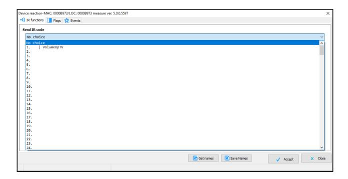
At the end, send the new list of conditions to the device. From now on, when the M-SERV input gets activated, an IR frame fetched from the remote control will be sent from the M-SENS module.
