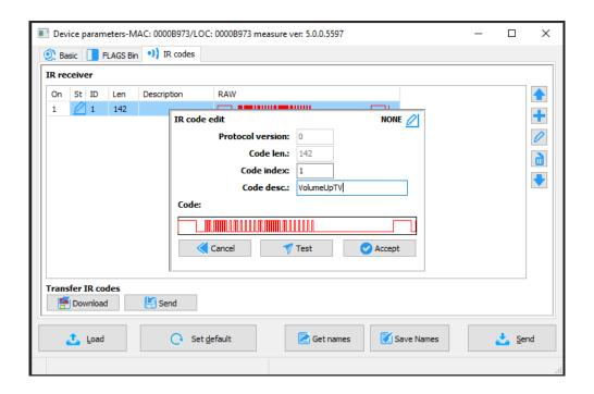
The next step is to confirm by clicking *Accept*. In order for the code to be saved in the device's memory, you have to click *Send* in the *Transfer IR codes* field. Once that is done, the status icon will look as follows:
