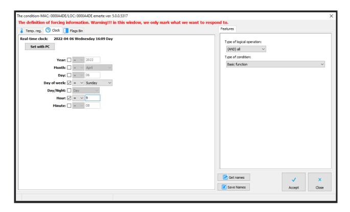
Select the output to which the pool cleaner pump is connected. Pick the Basic Function and Operation On. Confirm.
