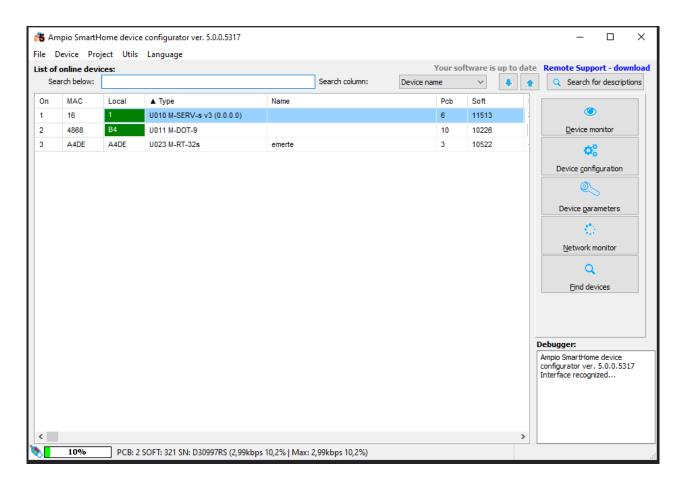
From the modules list, select *M-RT-s* and create a new condition from device.
