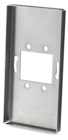
The guiding plate is designed for the installation of a touch panel. It is necessary for the correct assembly of the touch panel, providing that the panel's glass is as close to the wall as possible which ensures aesthetic look and no gap between the wall and the module. To achieve this, the guiding plate should be flush with the surface of the wall when fitted to the wall opening.
