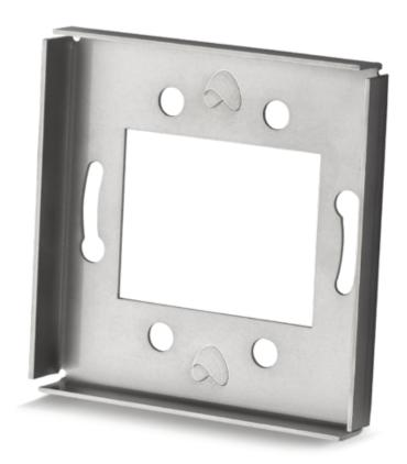
The guiding plate is designed for the installation of a touch panel. It is necessary for the correct assembly of the touch panel, providing that the panel's glass is as close to the wall as possible which ensures aesthetic look and no gap between the wall and the module. To achieve this, the guiding plate should be flush with the surface of the wall when fitted to the wall opening.
