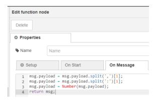
Different end devices can broadcast information in different ways, which is why it is worthwhile to view the data first in the *debug* window, before creating a function to send the information.
