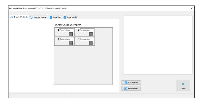
Apart from the simple on/off information, in the *Output values* tab you can also define a value per output within the range of 0-255 (which corresponds to 0-10V).
