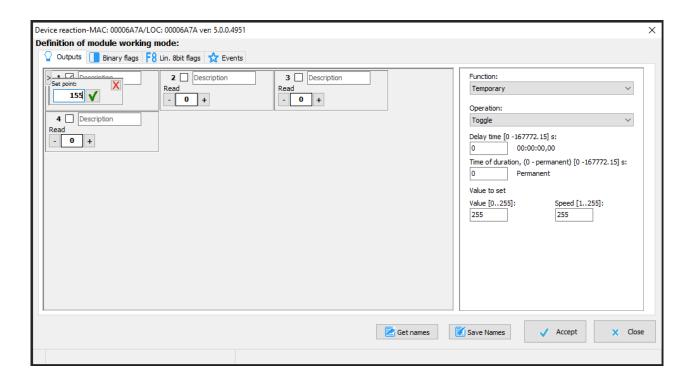
In the same window, on the right side, there is a list of functions that can be selected for a given condition, as well as the function parameters. Due to the fact that the module's outputs can not only be switched on/off, but also accept values in the range of 0-255, a lot of configuration possibilities are available.
