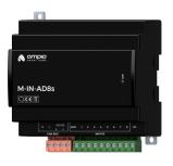
Supply voltage 11 - 16V DC Current consumption 190mA Number of analogue inputs 8 Analogue inputs impedance 20kΩ
