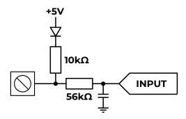
Generating a diagnostic signal within the power supply can be done in various ways. The module inputs are designed to work with potential-free relay outputs or optocoupler outputs. Before making the connection, check the documentation of the power supply to verify compatibility.
